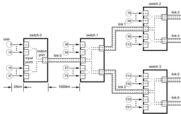
Figure 2: Network topology used in fairness simulations.
